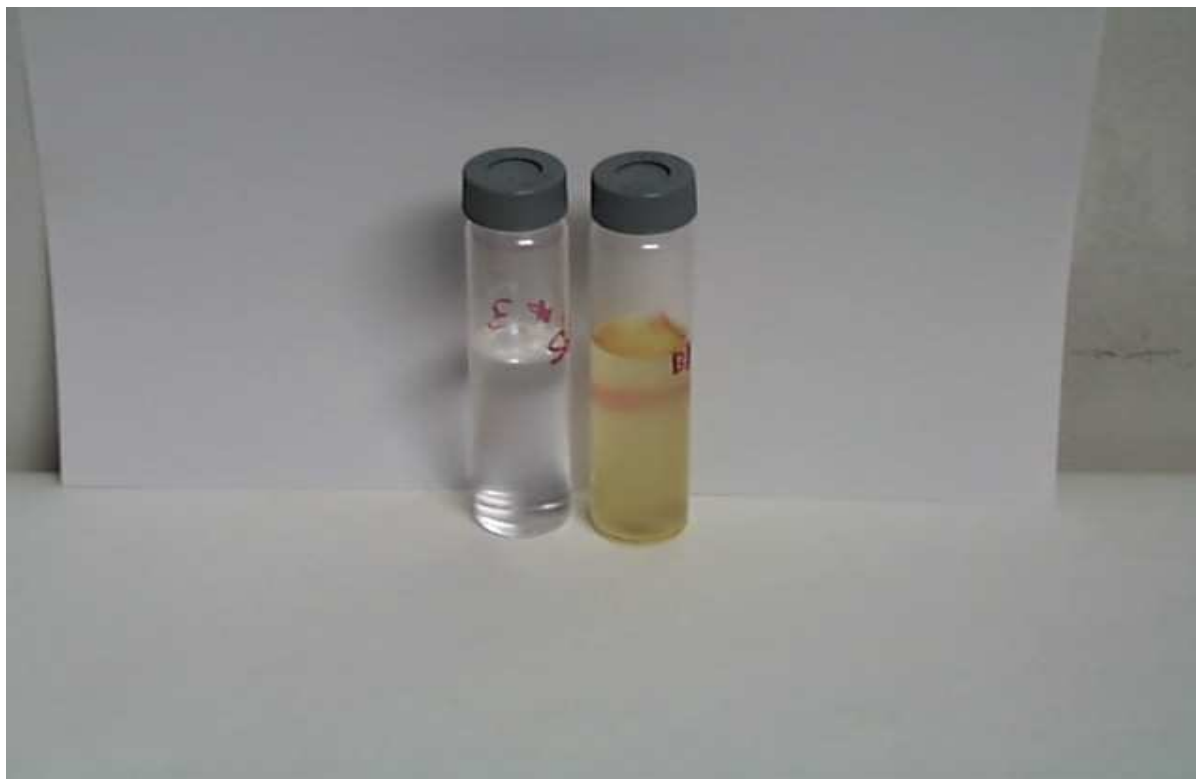
Extracts With and Without In-Cell Clean-Up of Fish Tissue Using Alumina, Silica Gel, and Acidic Silica Gel (40% H 2 SO 4 )
